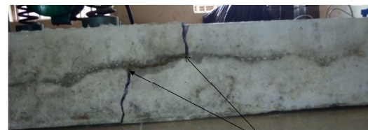
b: 1-fabric layer reinforced cement composite beam.
