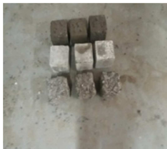
Figure 3. Cubes after chemical attack.
