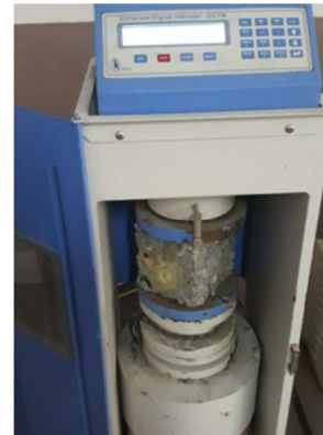
Figure 5. Compression test on cube.
