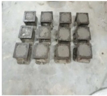
Figure 1. Casting of cube specimens.
